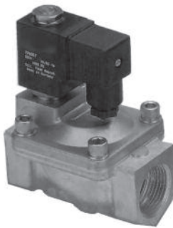
TB06HB-XXX-X Port Size: 3/4" NPT Orifice: 25 mm, 1" Cv: 12, SCFM: 336 Pressure Range: 10-150 PSI
