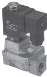
TB03EB-XXX-X Port Size: 3/8" NPT Orifice: 13 mm, 33/64" Cv: 4.5, SCFM: 126 Pressure Range: 10-150 PSI
